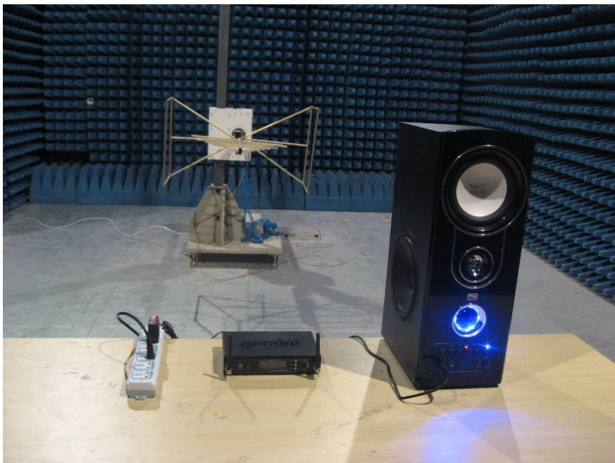
FCC RADIATED EMISSION TEST SETUP
