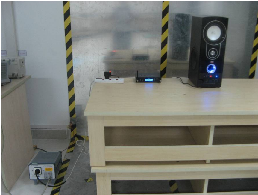
FCC LINE CONDUCTED EMISSION TEST SETUP
