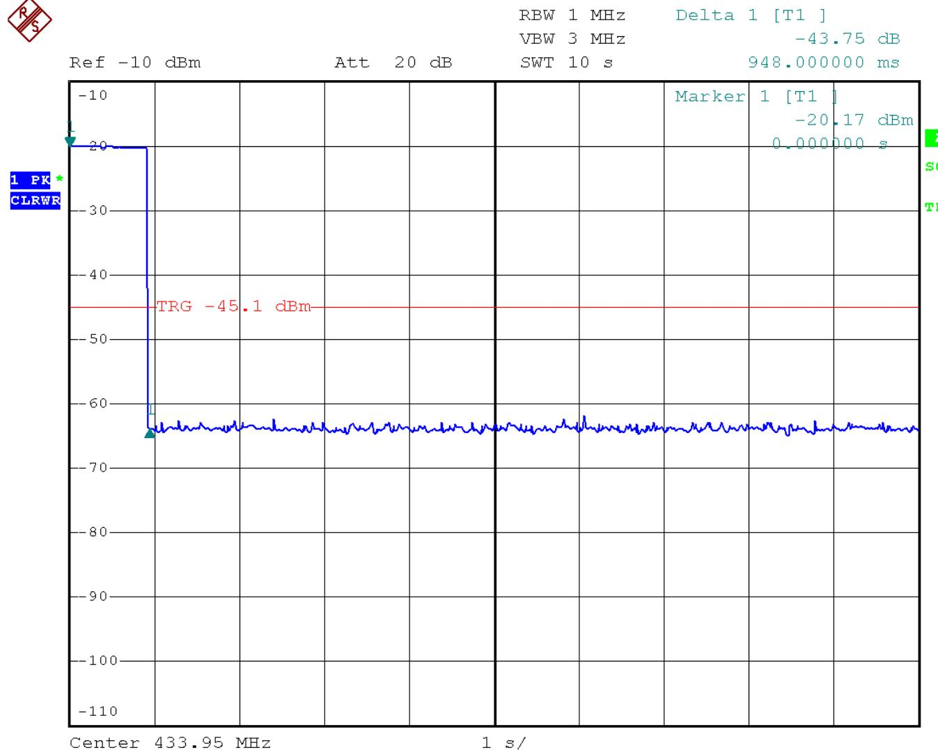
Timing Plot – Pursuant to FCC Part 15 Section 15. 231 Requirement
