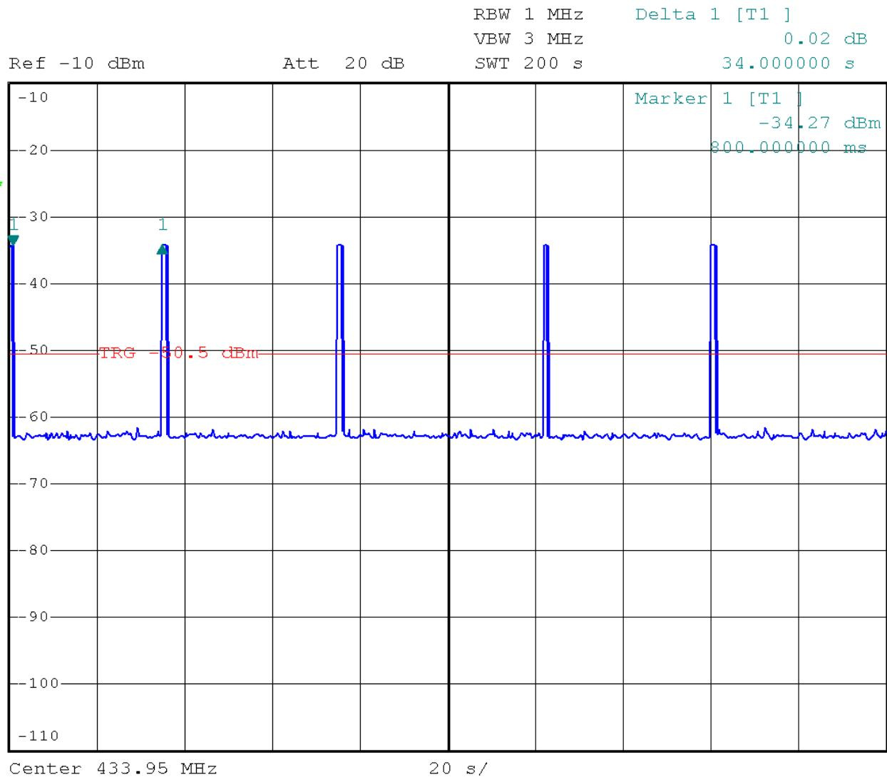
Timing Plot – Pursuant to FCC Part 15 Section 15. 231 Requirement
