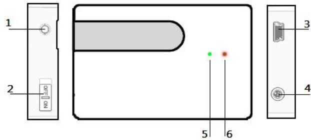
**1、ID key :** Building the connection between the dongle BOX and one or more speaker , and clear the interference
