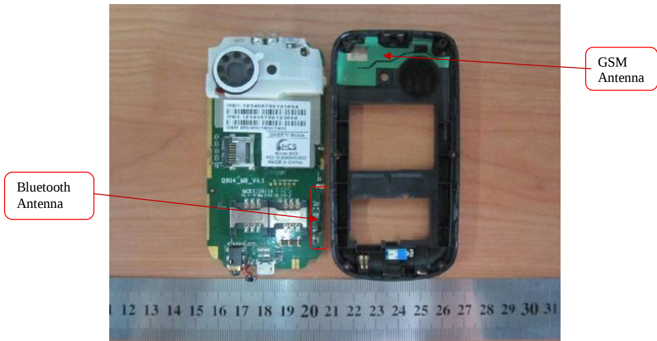
PCB Board view
