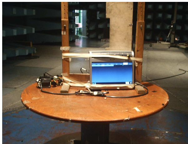
Log periodic antenna (30 MHz ÷ 1000 MHz) measurement distance: 3 m
