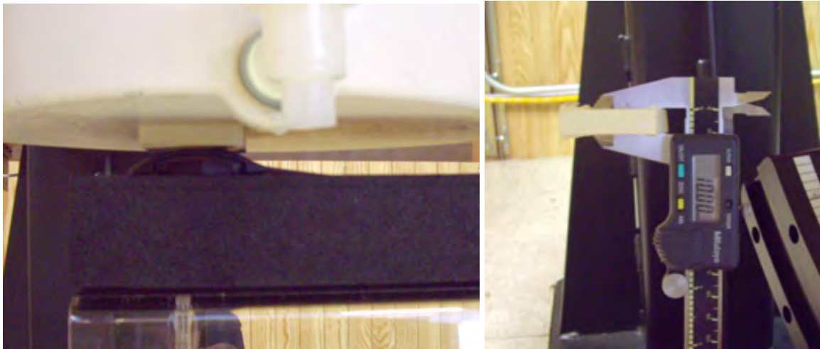
Figure 12-3 DUT front toward phantom, 1.0 cm separation, set-up photo
