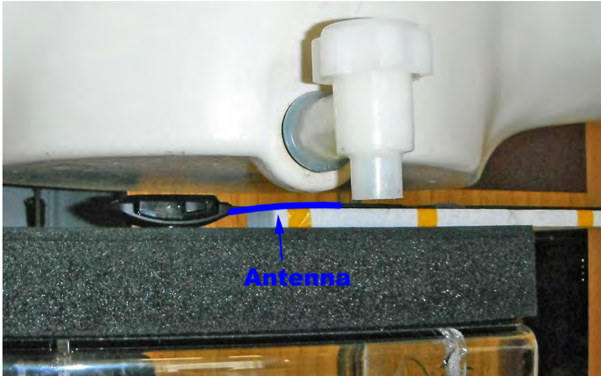
Figure 12-5 DUT rear toward phantom, 1.5 cm separation (spacing measurements were set up in similar fashion to that shown in Figure 12-4)
