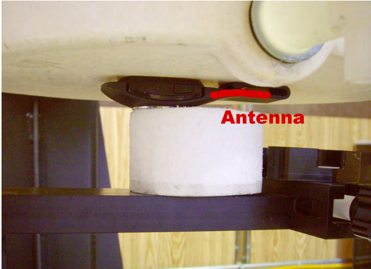
Figure 12-5 DUT rear toward phantom, 0 cm separation (spaced measurements were set up in similar fashion to that shown in Figure 12-4)
