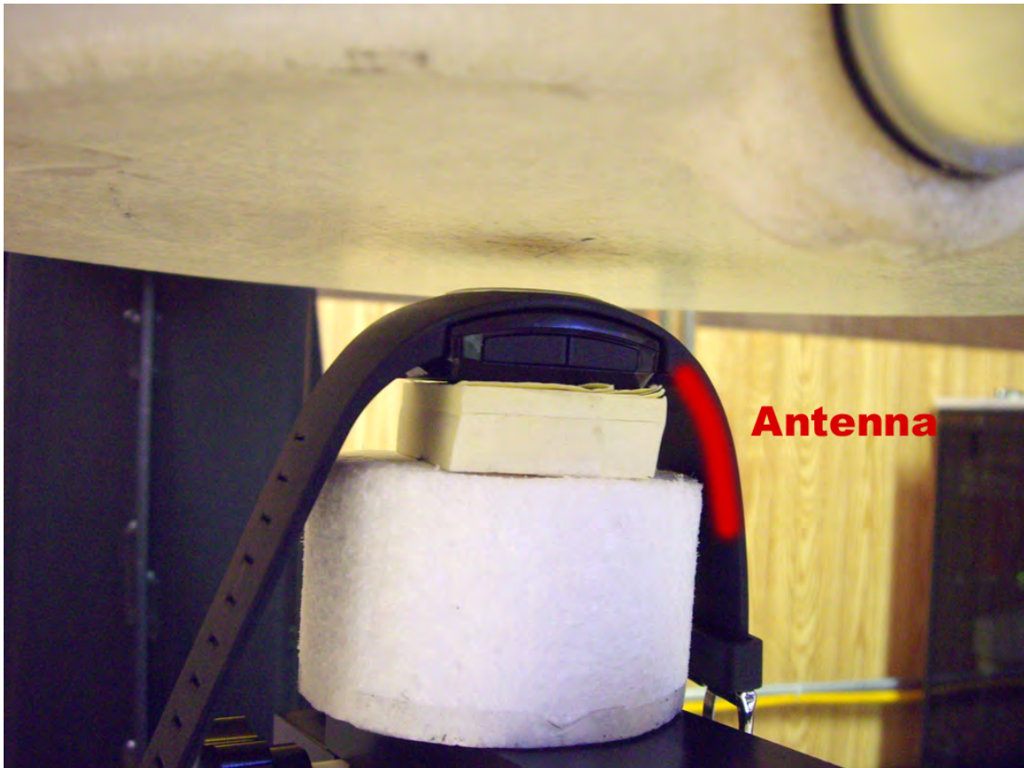
Figure 12-5 DUT front toward phantom, 1.0 cm separation, as tested
