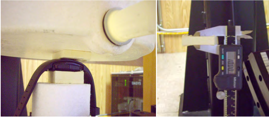
Figure 12-4 DUT front toward phantom, 1.0 cm separation, set-up photo
