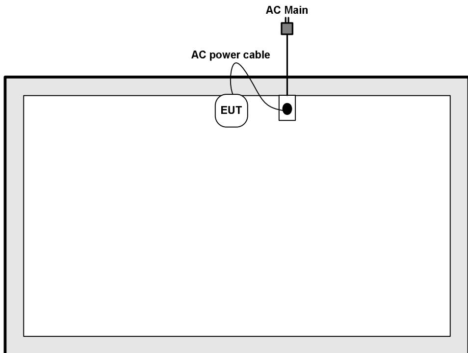
**Test Setup Diagram - Radiated Test (Above 1GHz)**
