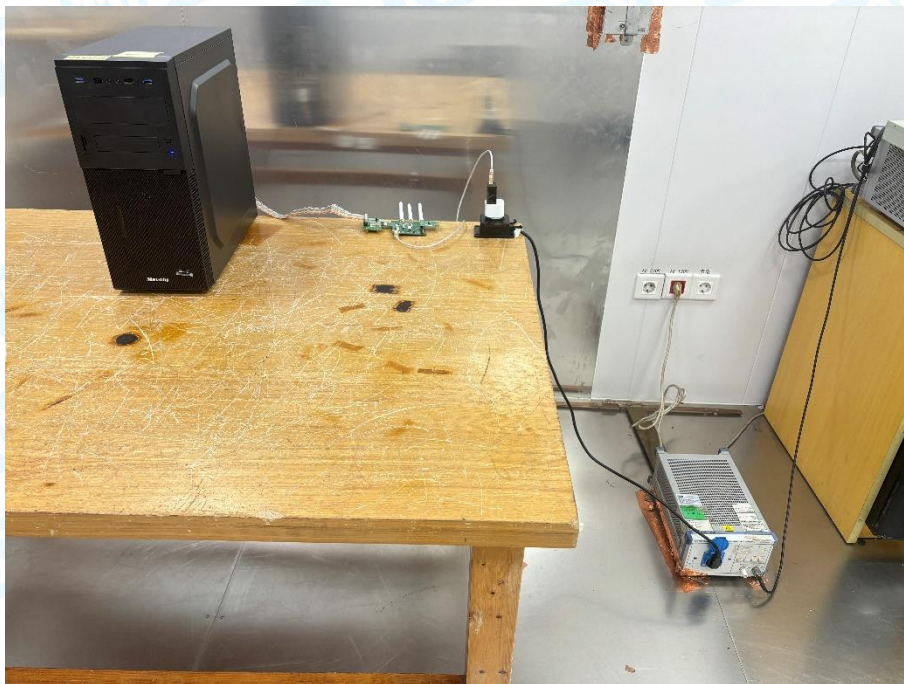
Photo of Setup for Conducted Emission
