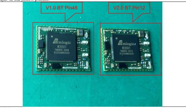
BT Port pin48 (Resistor placement R7) BT Port pin12 (Resistor placement R8)
