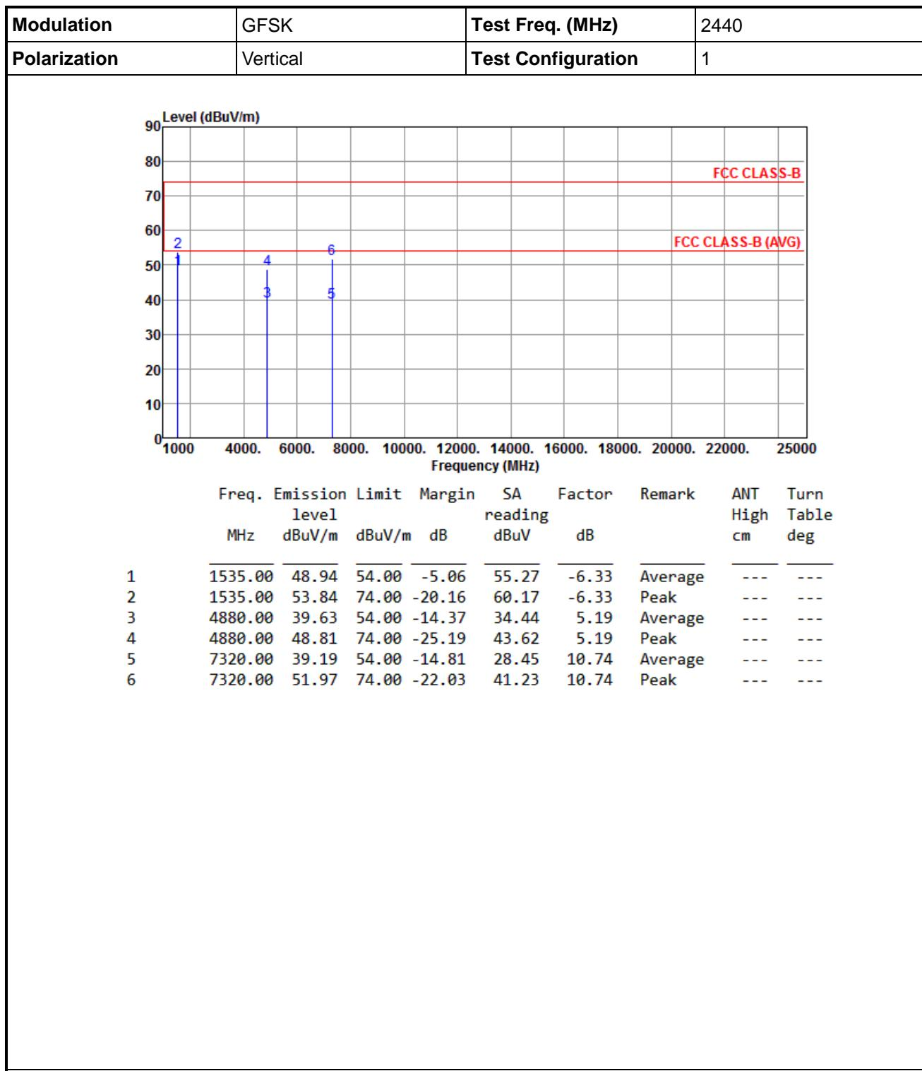
Note 1: Emission Level (dBuV/m) = SA Reading (dBuV/m) + Factor\* (dB)
