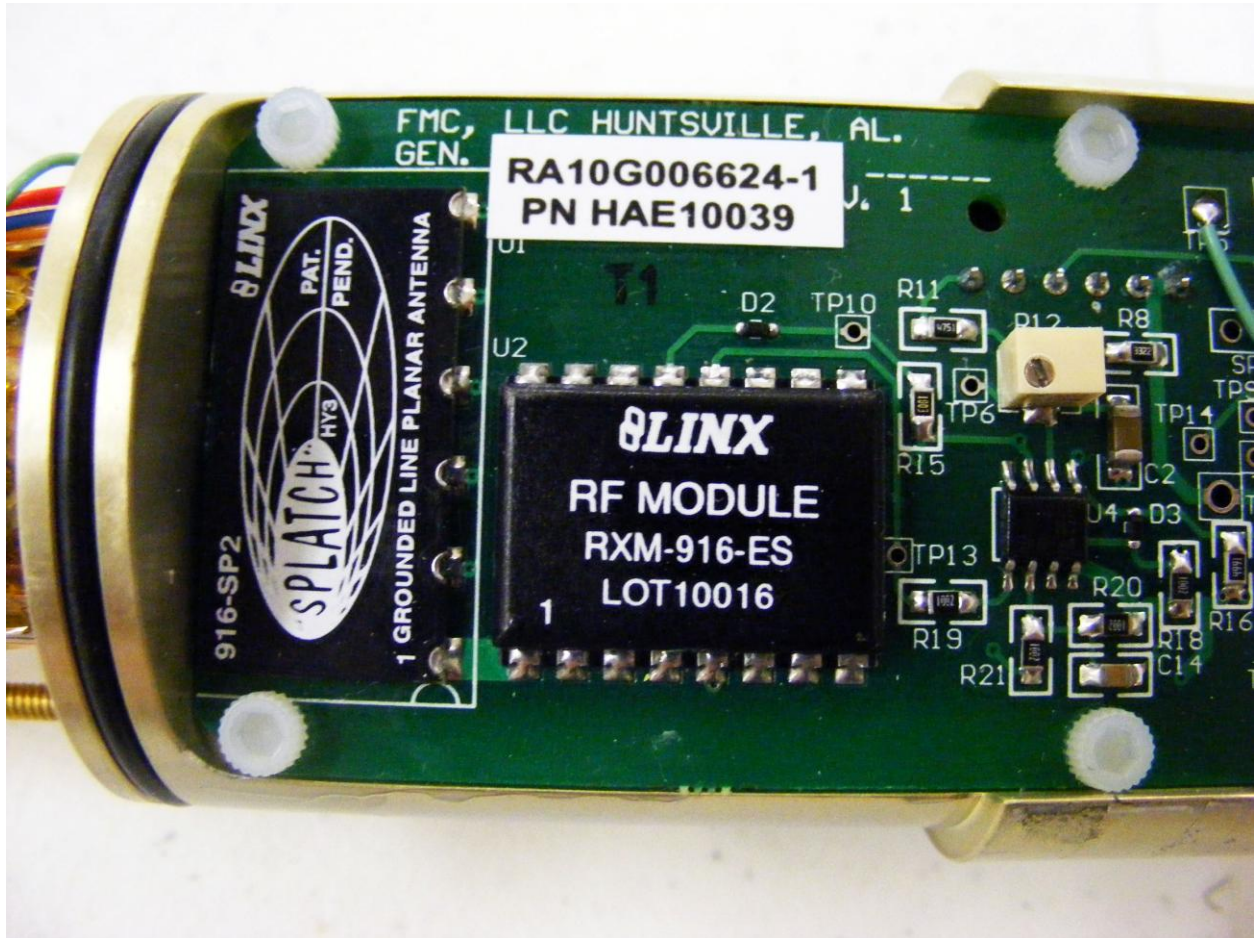
Underground Proximity Generator – Internal Photo RF Receiver Module and Antenna
