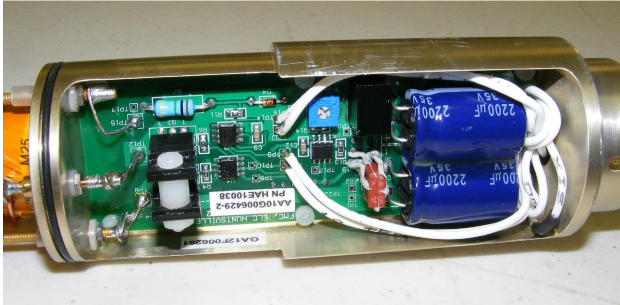
Underground Proximity Module – Internal Photo Amplifier Circuit Board – Bottom Side
