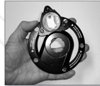
5. Shift the large chainring onto the battery compartment.
