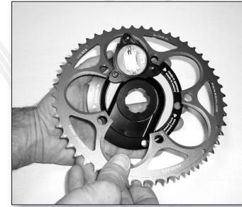
6. Bring the holes for the threaded connections in line.
