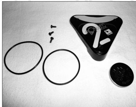
2. Mount the O-rings. Insert the smaller one into the battery cover.
