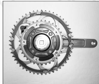
Crank mounting example: SRAM comp. variant
