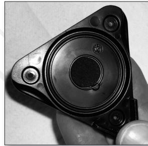
3. Place the larger O-ring around the upper collar of the battery compartment as shown in the figures.
