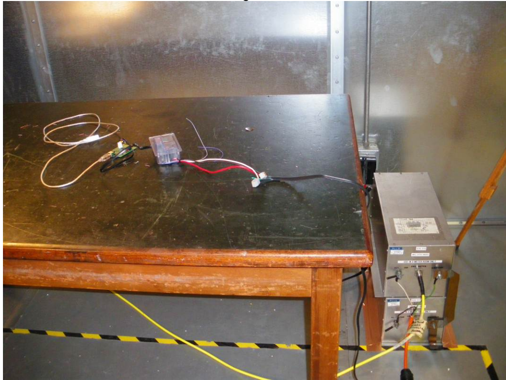
Test Set-up for Conducted Emissions
