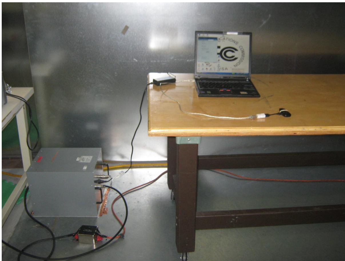
Figure 2 – Power line conducted emissions
