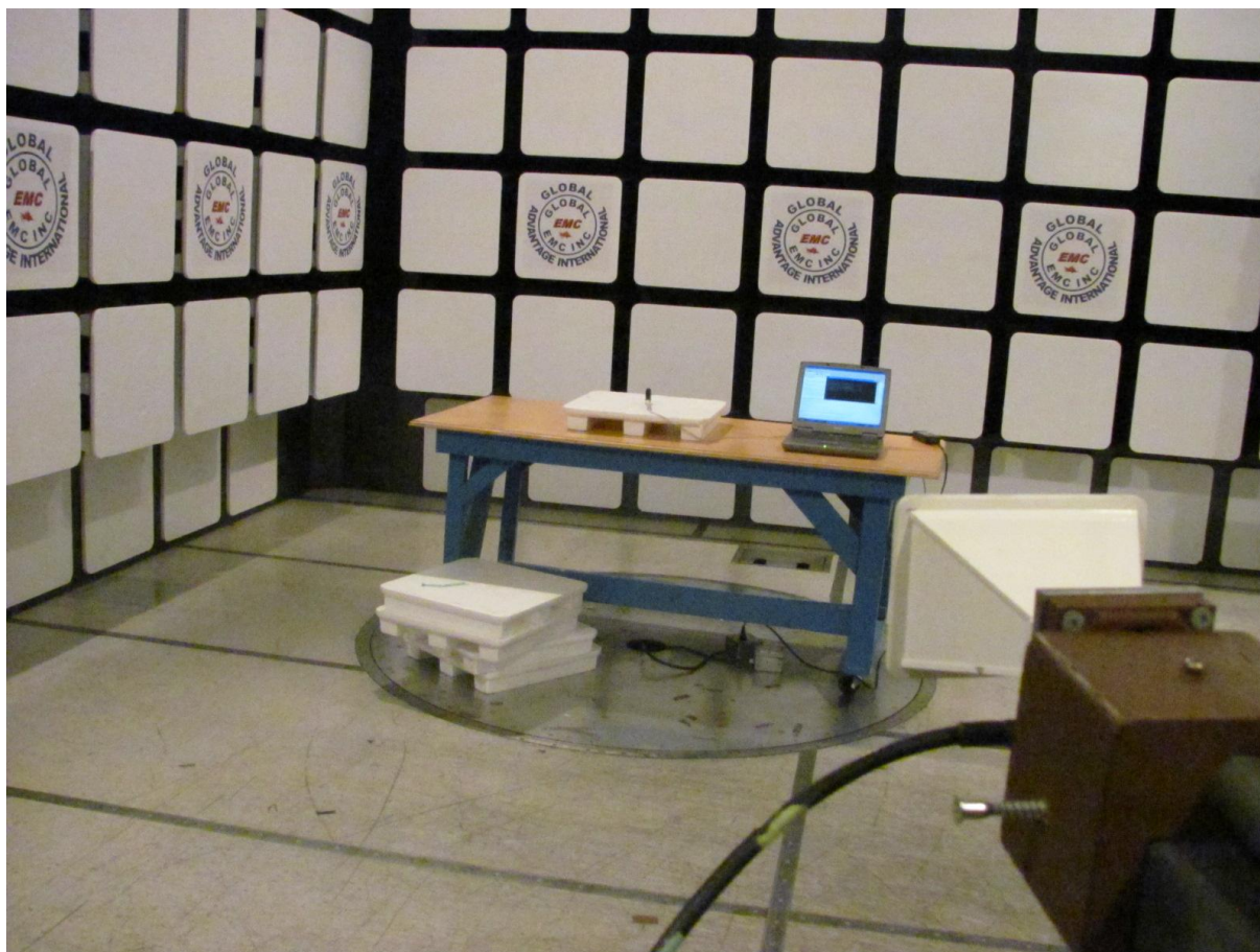
Figure 1 – Radiated emission setup
