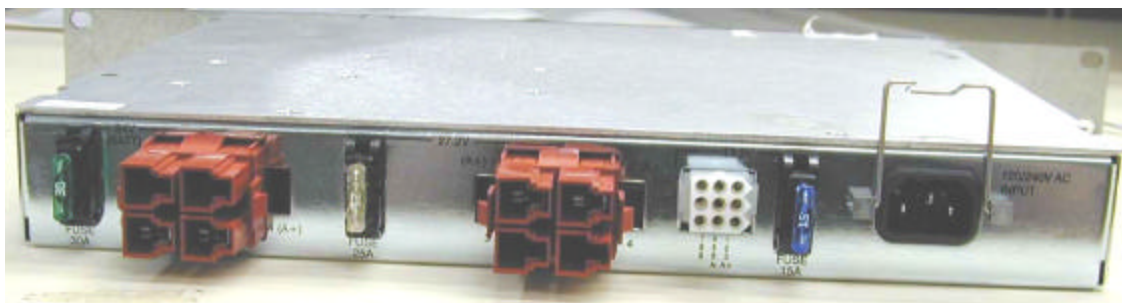
Figure 3: AC/DC Power Supply Back Connectors
