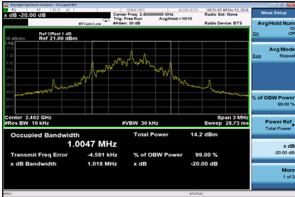
**20dB Bandwidth Test Data CH-Mid**
