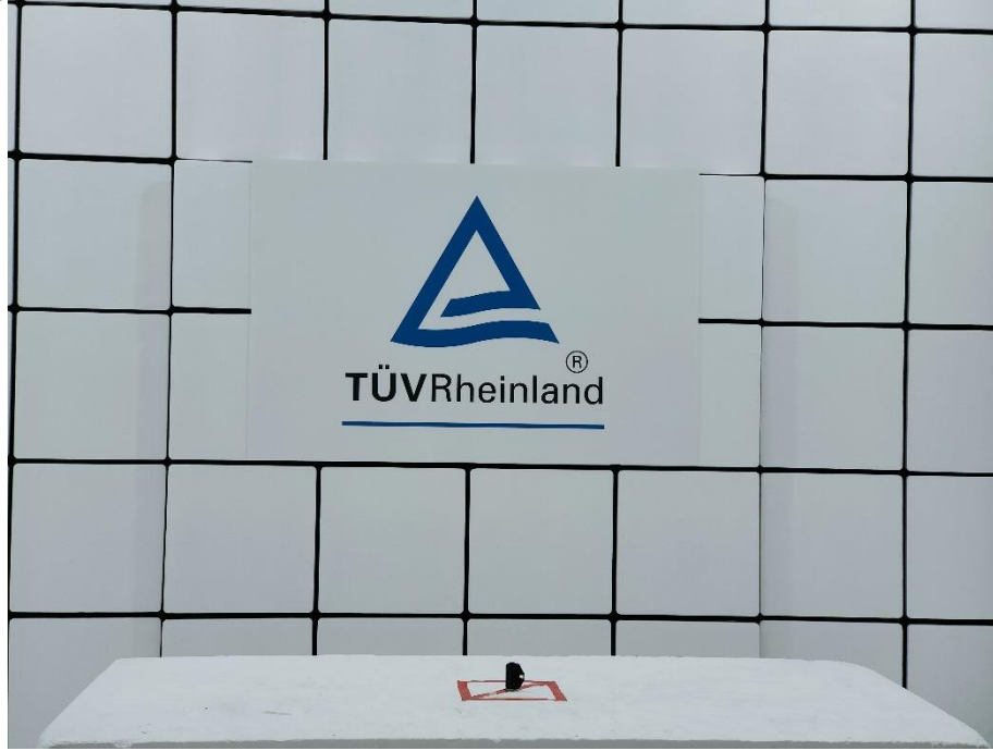
Photograph 8: Test Setup for Spurious Emissions (Front View 2, FSK Mode)
