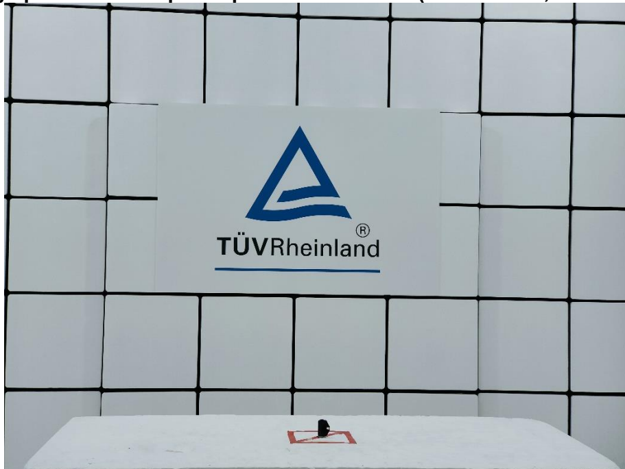
Photograph 2: Test Setup for Spurious Emissions (Front View 2, ASK Mode)
