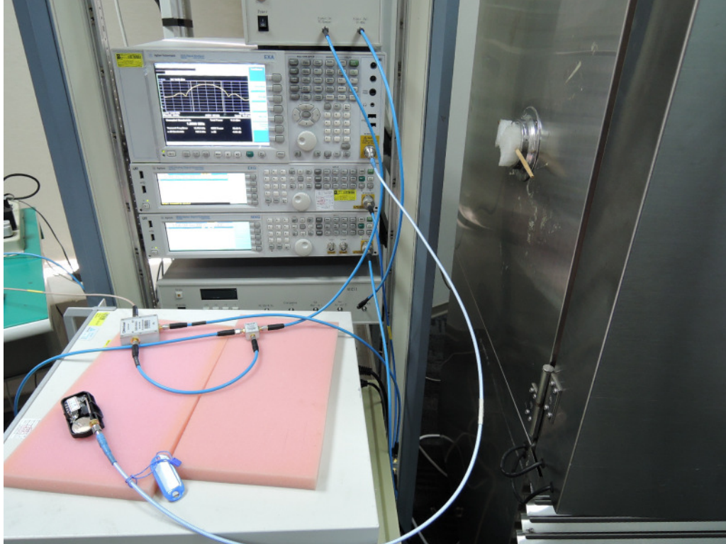
Photograph 6: Set-up for Conducted testing
