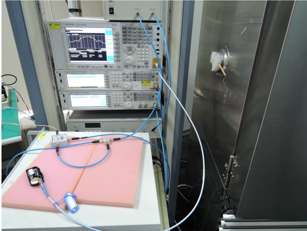
Photograph 6: Set-up for Conducted testing
