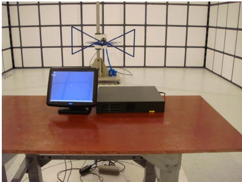
Maximized Radiated Emission Test Set-up View
