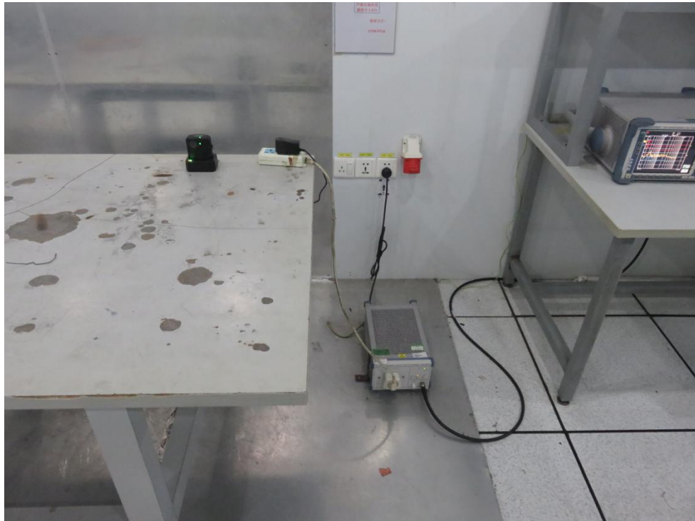
Photo of Conducted Emission Measurement
