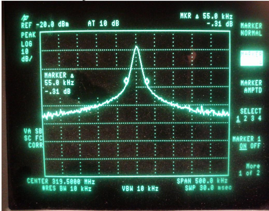
Bandwidth of the modulated signal is 55 kHz
