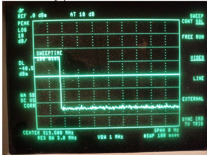
Plot below shows an expanded view of the transmitted packet.
