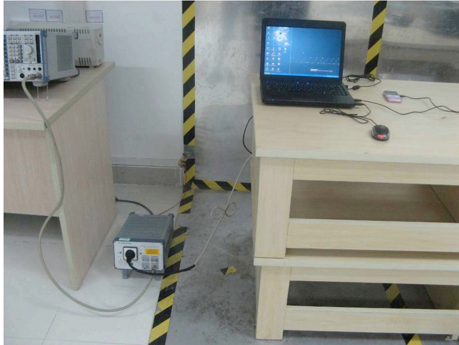
FCC LINE CONDUCTED EMISSION TEST SETUP
