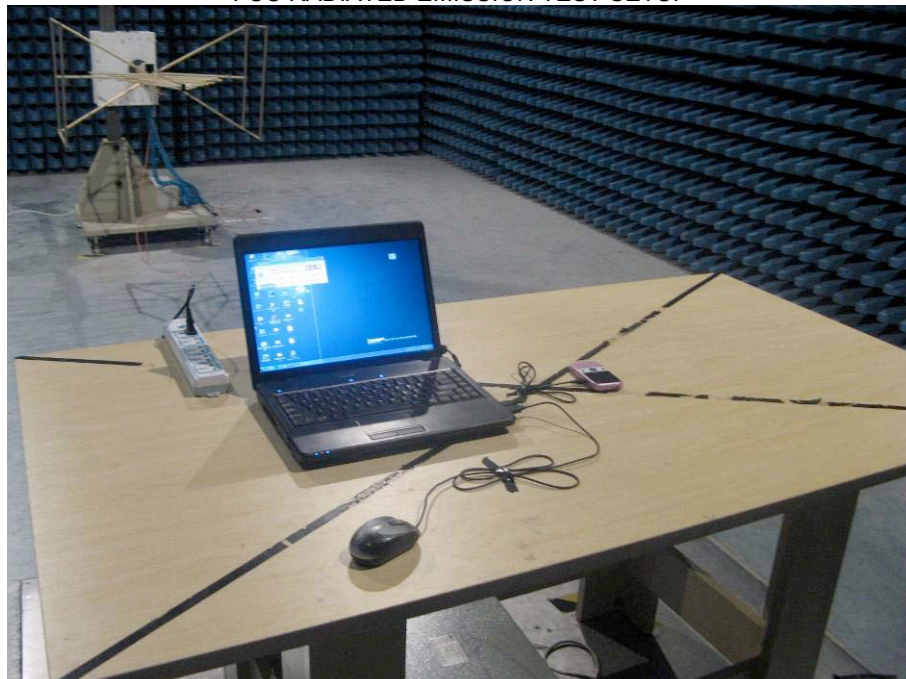
FCC RADIATED EMISSION TEST SETUP
