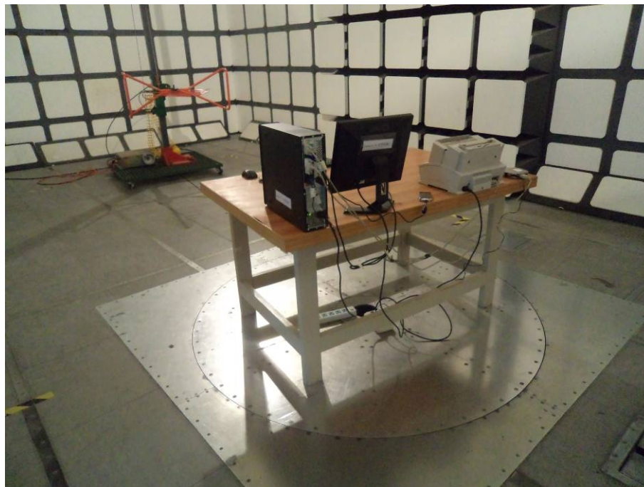
Radiated Emissions - Rear View (downloading mode)
