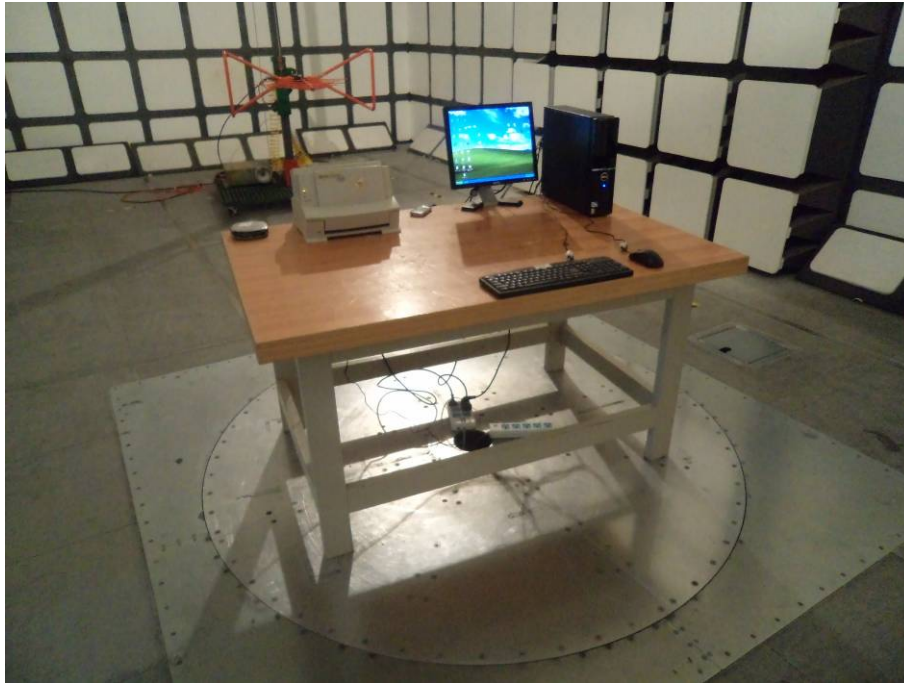
Radiated Emissions - Front View (downloading mode)
