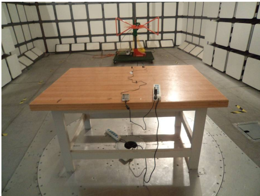
Radiated Emissions –Rear View (charging & media playing mode)
