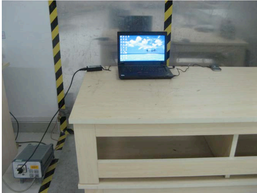
FCC LINE CONDUCTED EMISSION TEST SETUP
