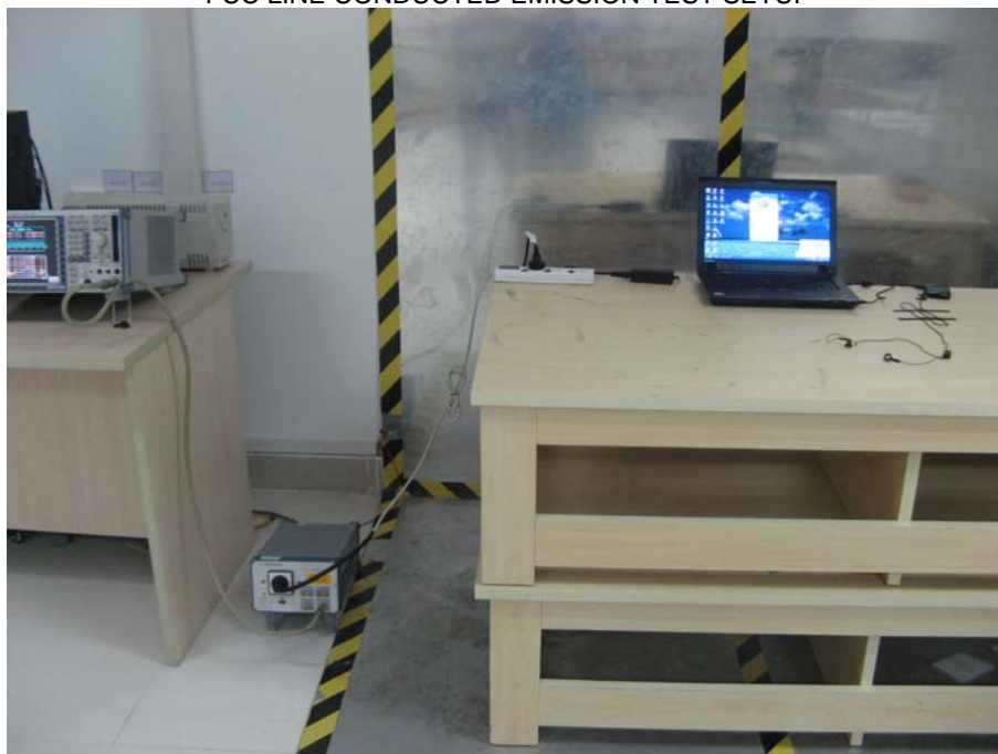
FCC LINE CONDUCTED EMISSION TEST SETUP
