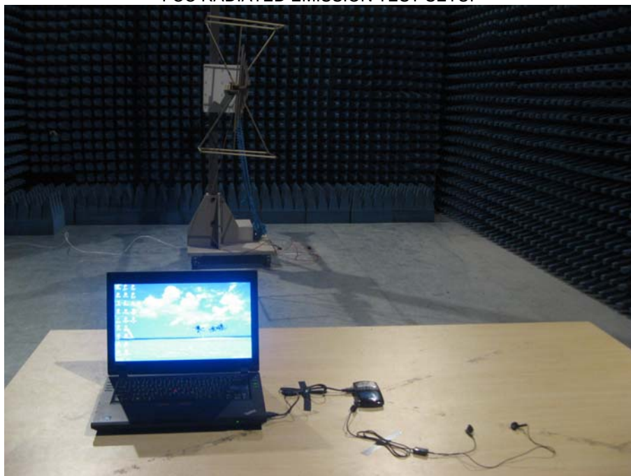
FCC RADIATED EMISSION TEST SETUP
