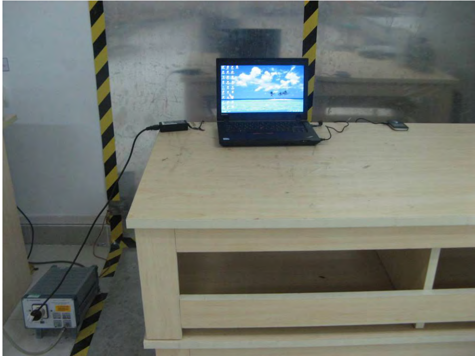
FCC LINE CONDUCTED EMISSION TEST SETUP
