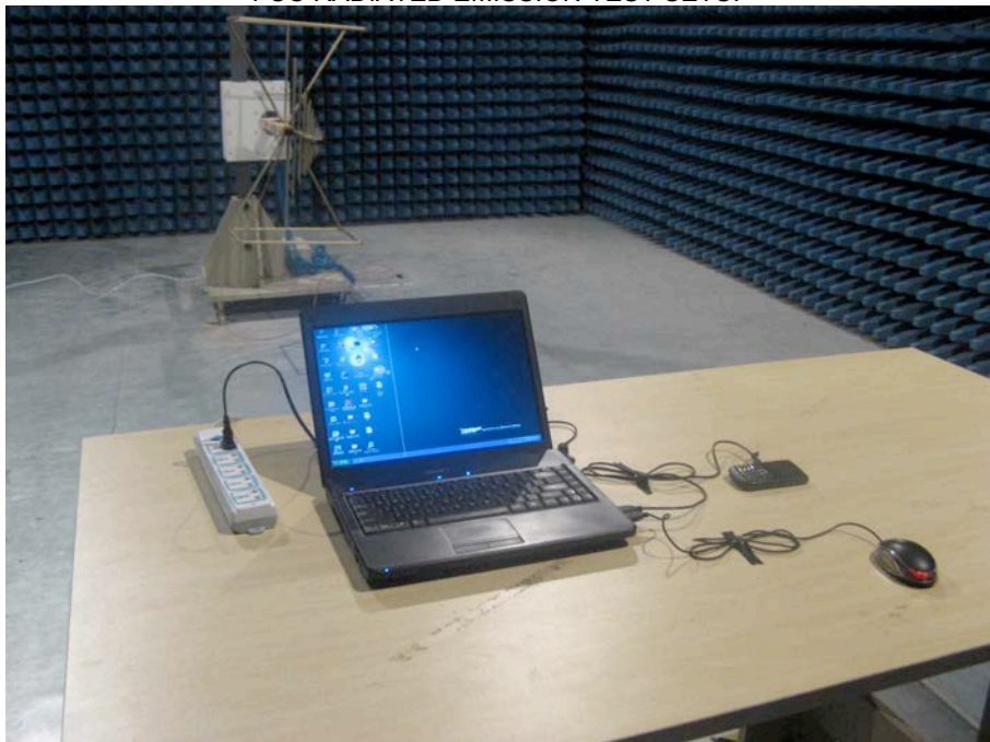
FCC RADIATED EMISSION TEST SETUP
