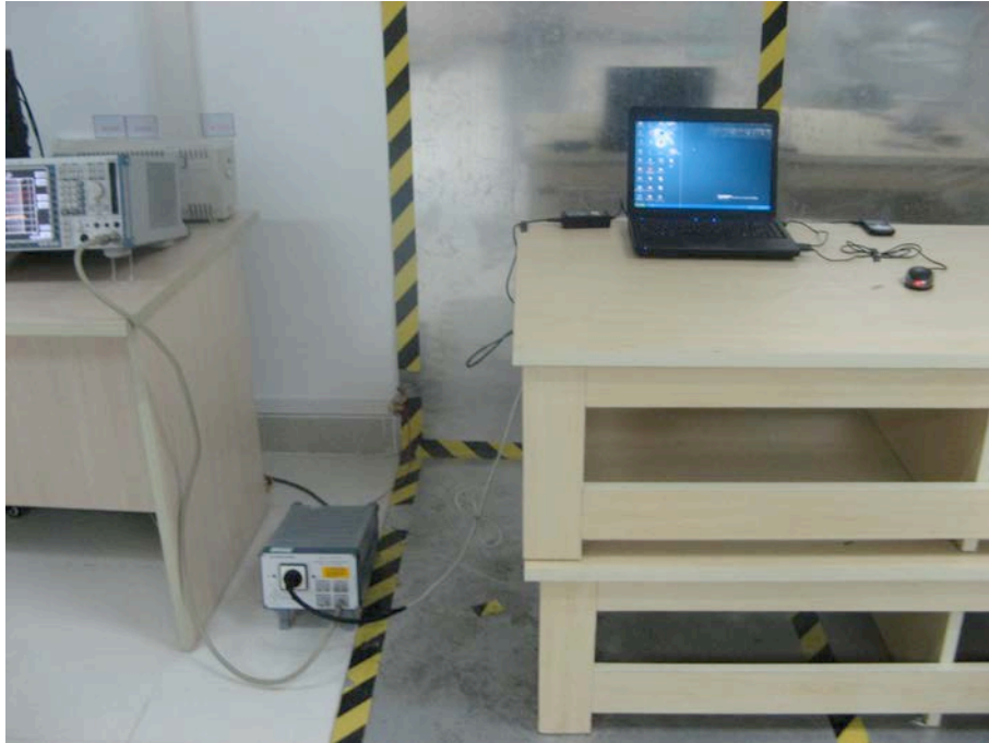
FCC LINE CONDUCTED EMISSION TEST SETUP
