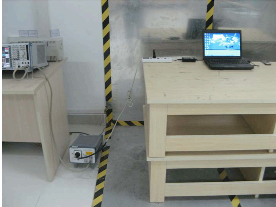
FCC LINE CONDUCTED EMISSION TEST SETUP
