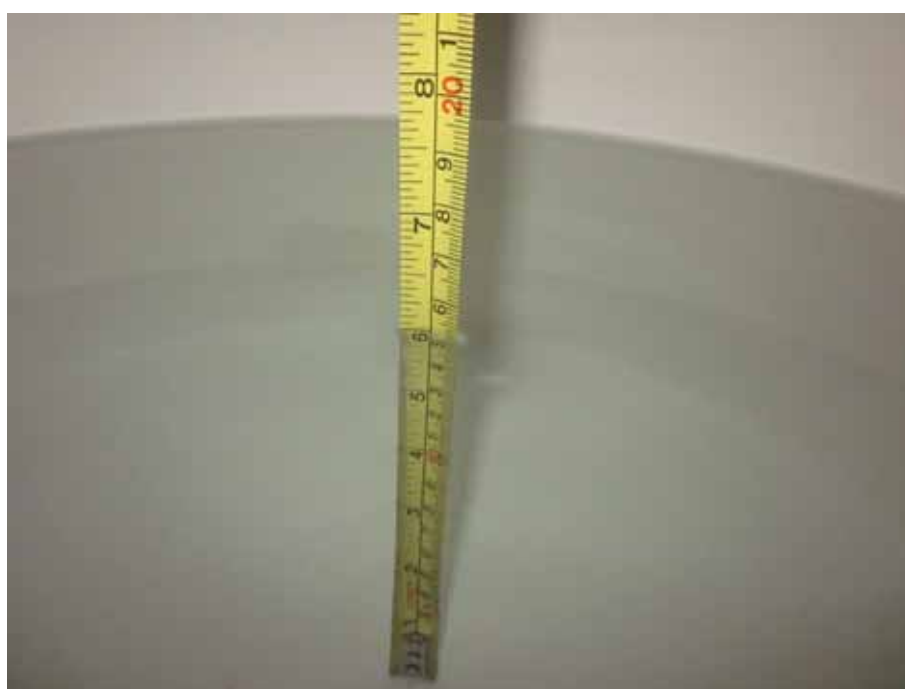
Figure 10.2: Liquid depth in the Flat Phantom ( 835MHz, 1900MHz 15.2cm)
