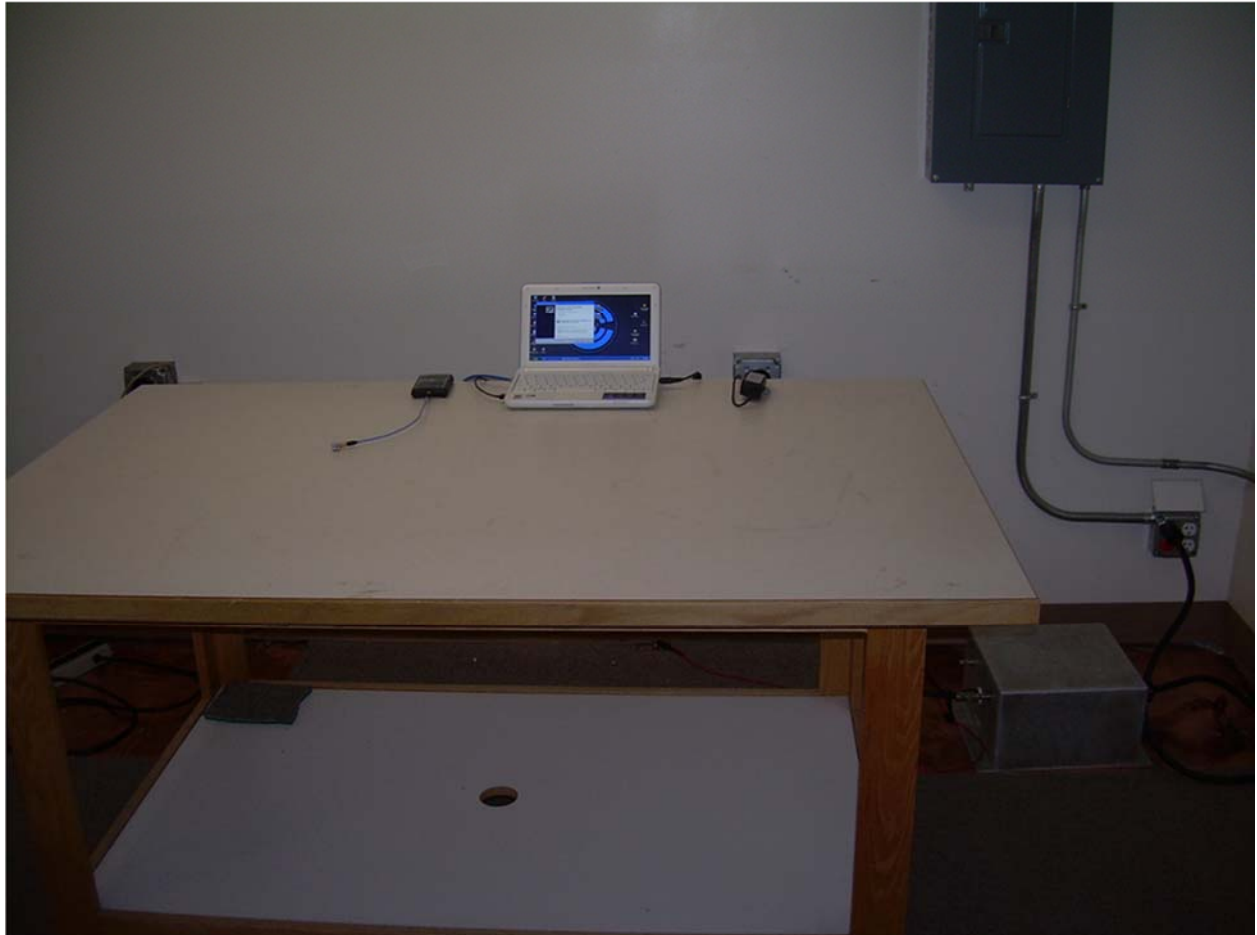
Front View Conducted Disturbance Worst Case Configuration
