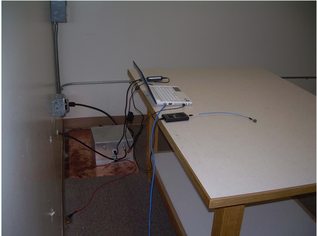
Back View Conducted Disturbance Worst Case Configuration
