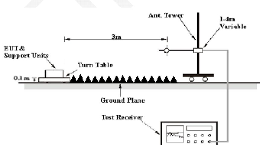
The radiated emission and out of band emission tests were performed in the 3 meters chamber test site, using the setup accordance with the ANSI C63.4-2003. The specification used was the FCC 15.209/15.205 and FCC 15.249 limits.
