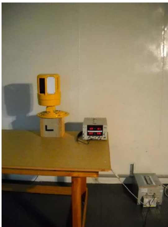
Photograph 7.6.1 Setup for conducted emission measurements
