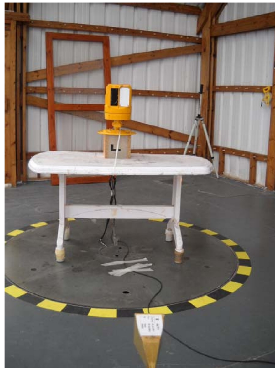
Photograph 7.5.1 Setup for occupied bandwidth measurements
