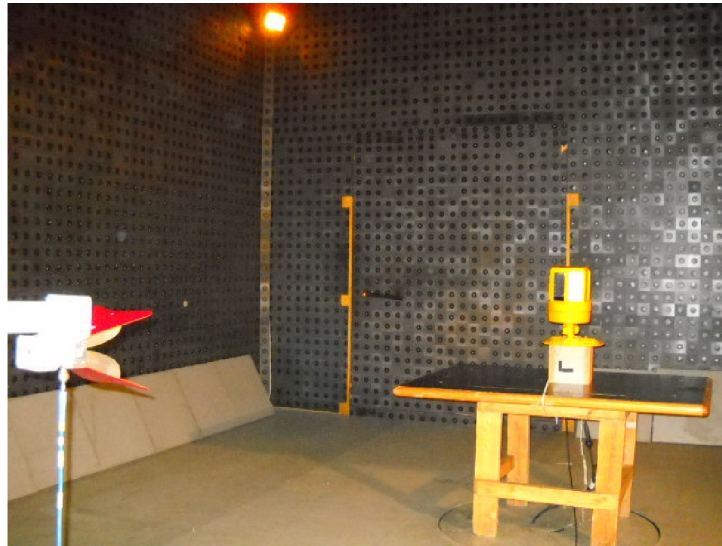
Photograph 7.2.3 Setup for radiated emissions measurements above 1000 MHz
