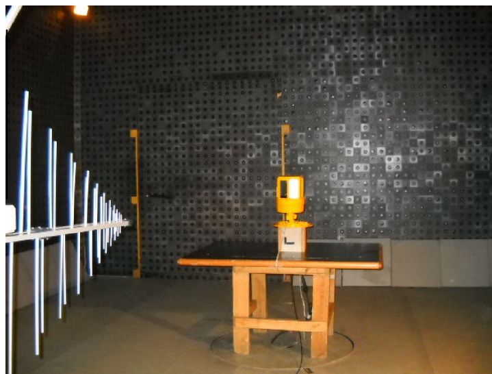
Photograph 7.2.2 Setup for radiated emissions measurements above 30 MHz
