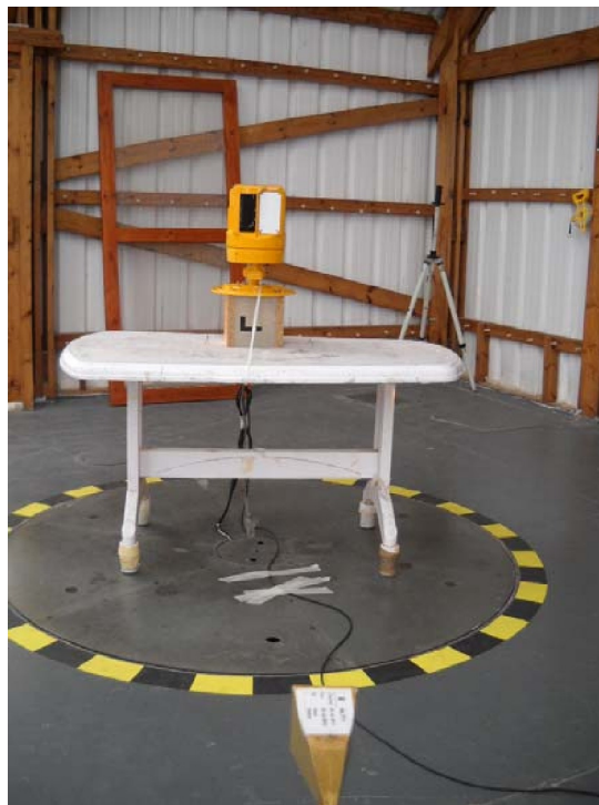
Photograph 7.1.1 Setup for in band radiated emission measurements
