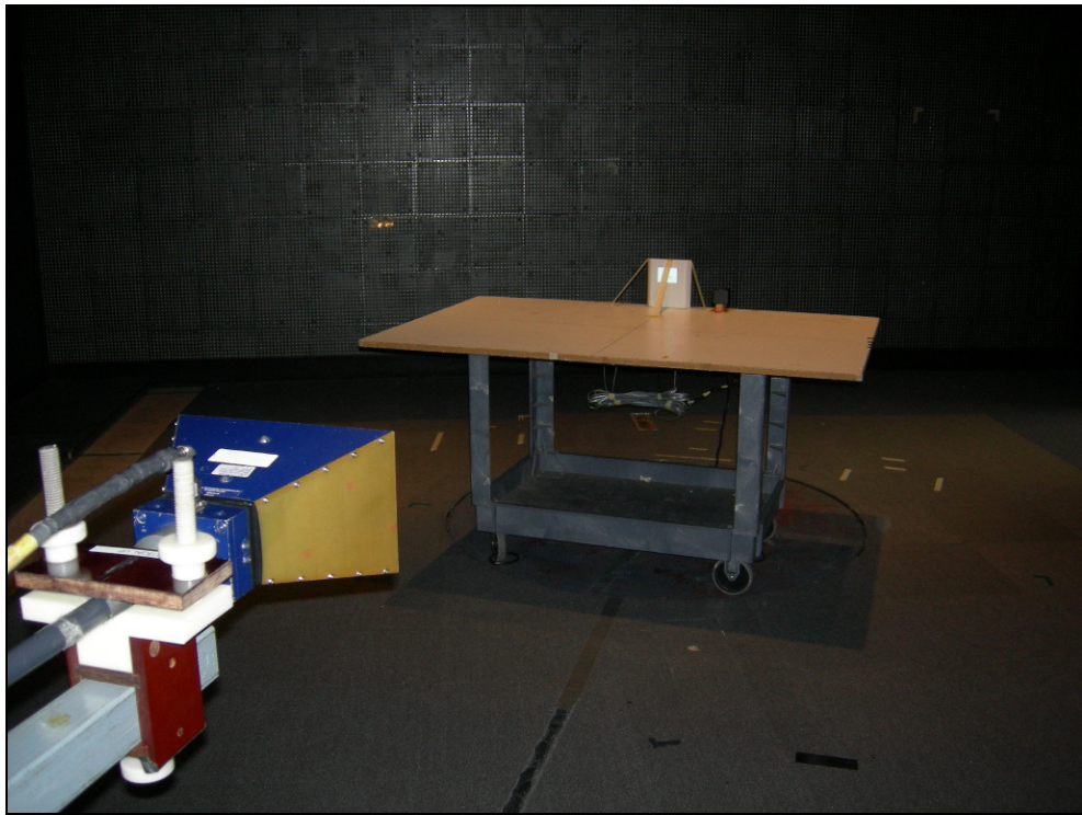
Figure 3: Radiated Emissions with Power Supply
