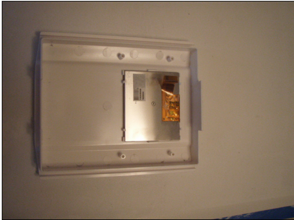
Figure 3: PCB Removed and Display Installed
