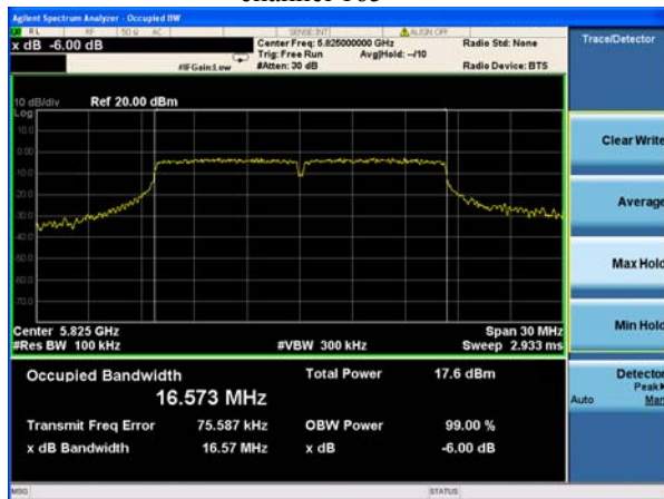
(802.11a) -6dB Bandwidth plot on channel 165
