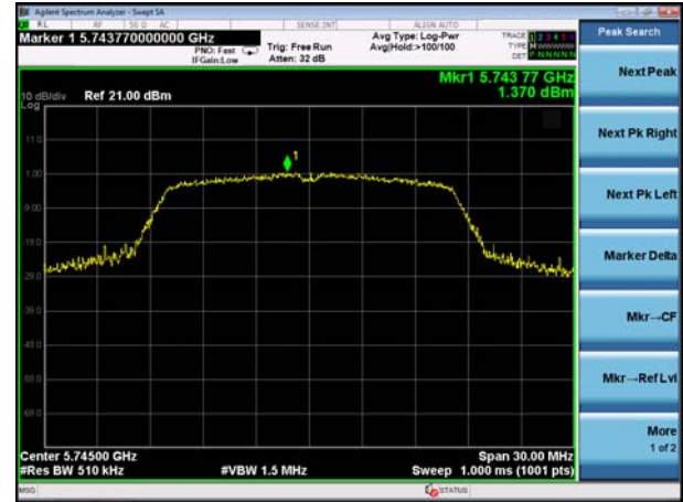
(802.11n20) PSD plot on channel 149
