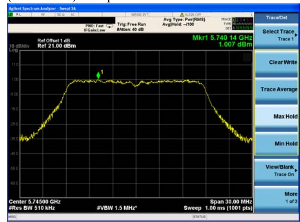
(802.11ac20) PSD plot on channel 149
