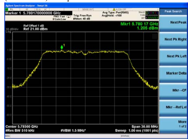
(802.11ac20) PSD plot on channel 157
