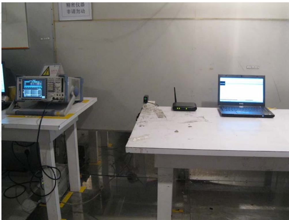
TEST SETUP OF CONDUCTED EMISSION (front view)
