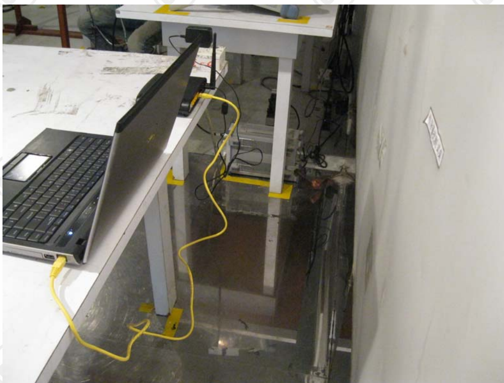
TEST SETUP OF CONDUCTED EMISSION (side view)
