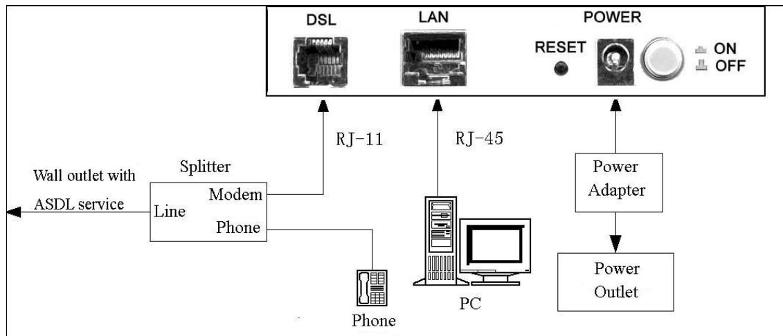
**Notes:** Without the splitter and certain situation, transient noise from telephone can interfere with the operation of the ADSL router, and the ADSL router may introduce noise to the telephone line. To prevent this from happening, a small external splitter must be connected to each telephone.
