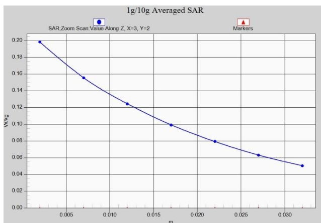
Fig. 1-1 Z-Scan at power reference point (850 MHz)
