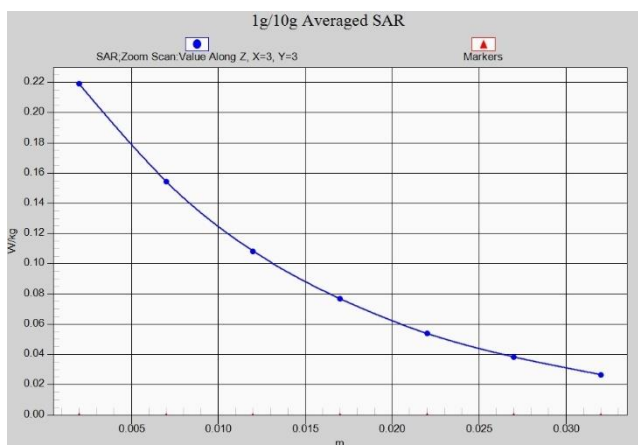
Fig. 1-7 Z-Scan at power reference point (WCDMA1700)
