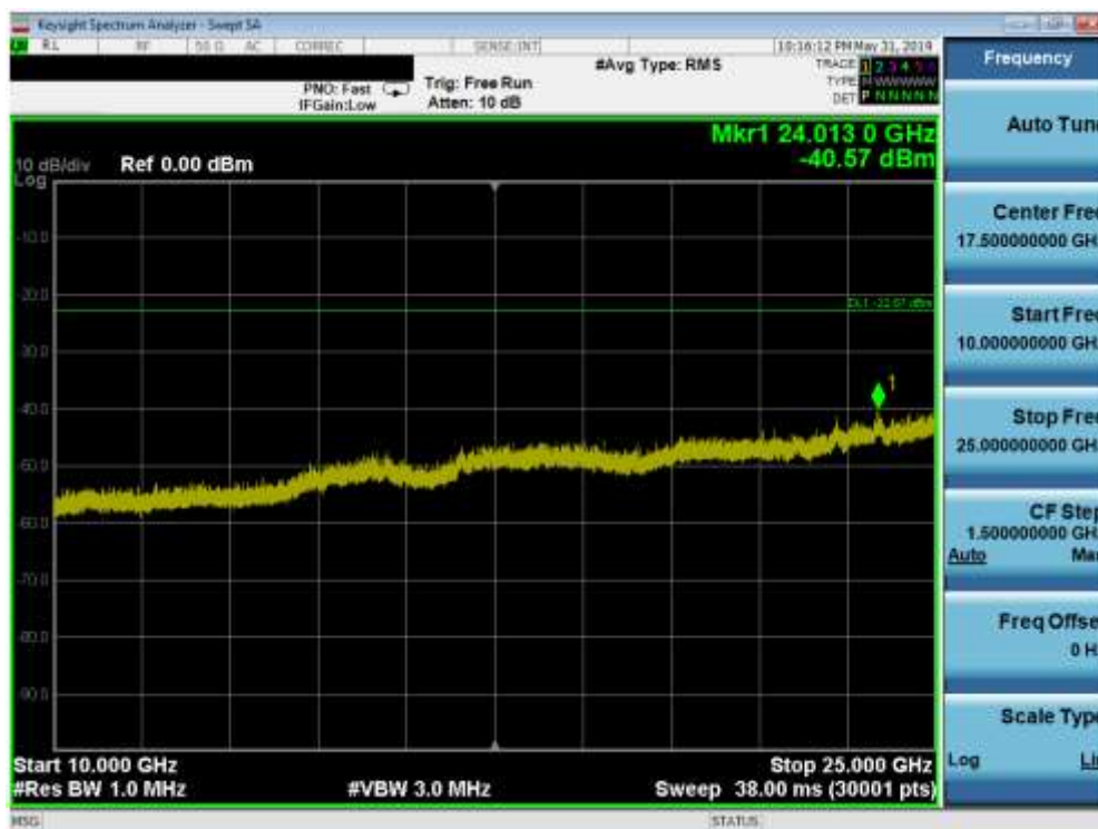
Plot 7-26. Conducted Spurious Plot (802.11b – Ch. 1)
