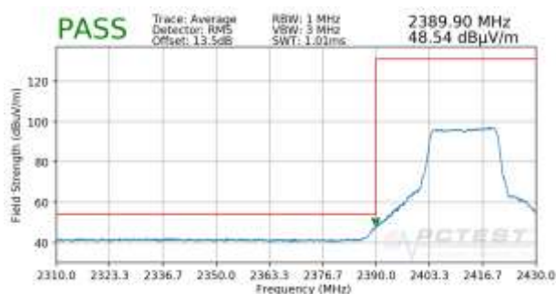
Plot 7-35. Radiated Restricted Lower Band Edge Measurement (Average)
