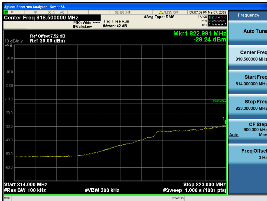
LTE Band 5 / 10MHz / QPSK - RB Size/Offset (25/0)
