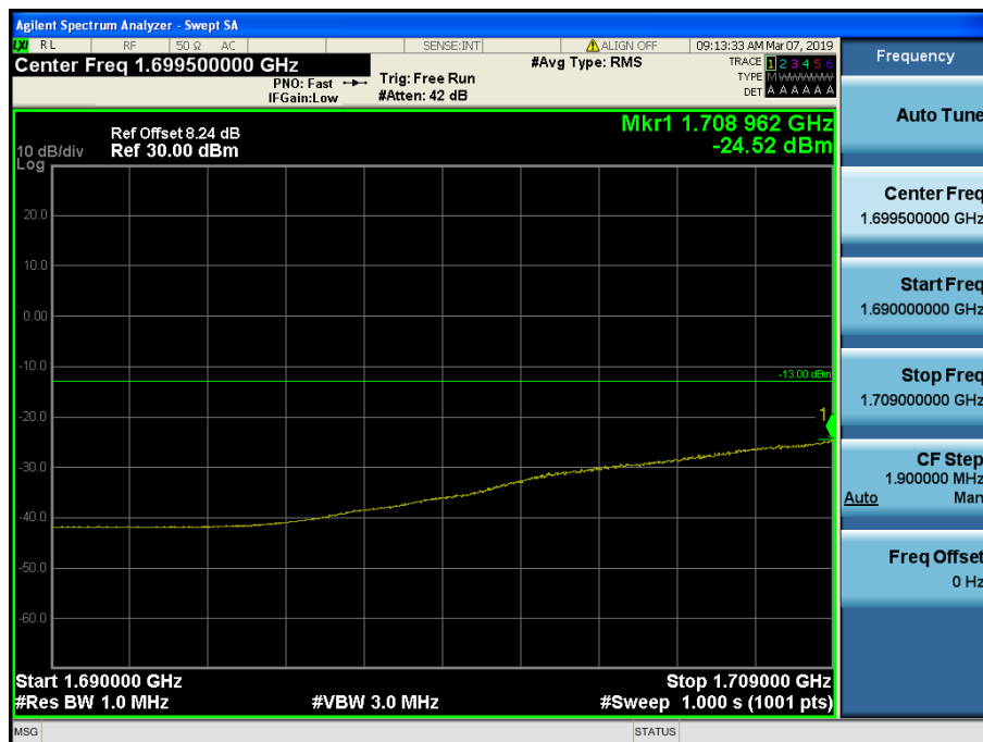
LTE Band 66, 4 / 20MHz / QPSK - RB Size/Offset (50/0)
