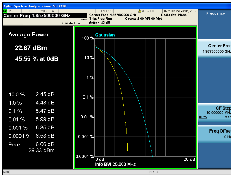
LTE Band 2 / 15 MHz / QPSK - RB Size 75
