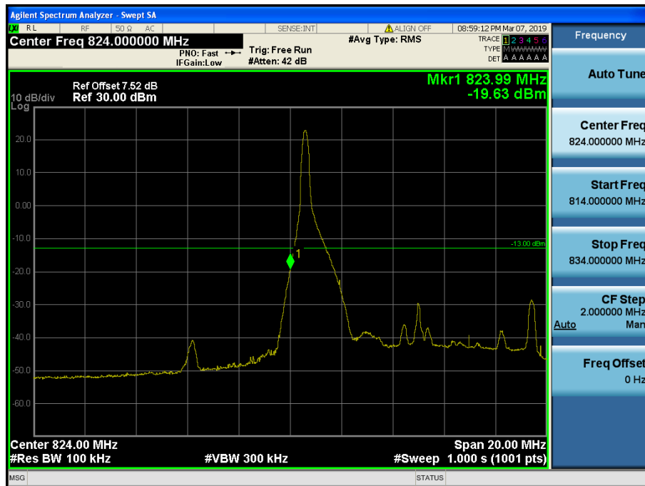
LTE Band 5 / 10MHz / QPSK - RB Size/Offset (1/0)
