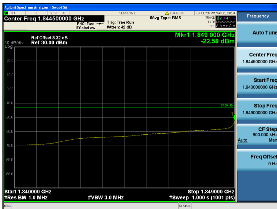
LTE Band 2 / 10MHz / QPSK - RB Size/Offset (25/0)
