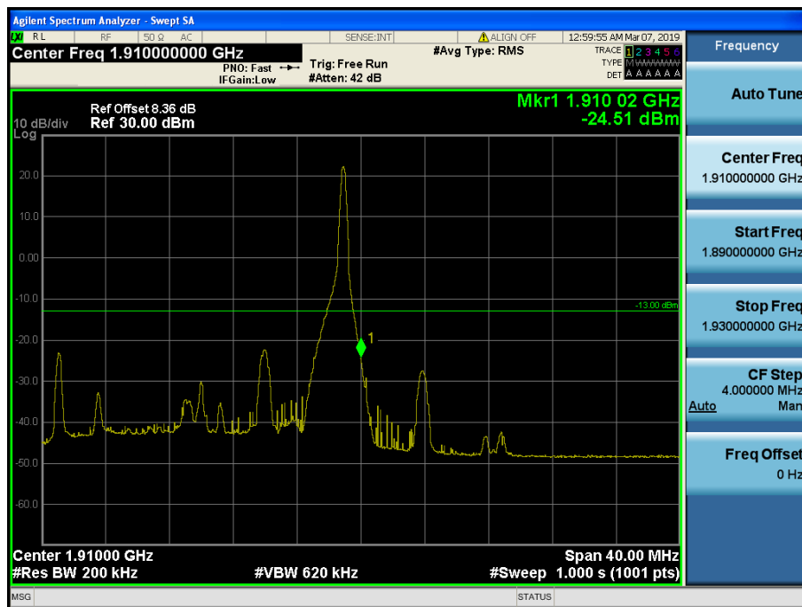
LTE Band 2 / 20MHz / 16QAM - RB Size/Offset (1/99)
