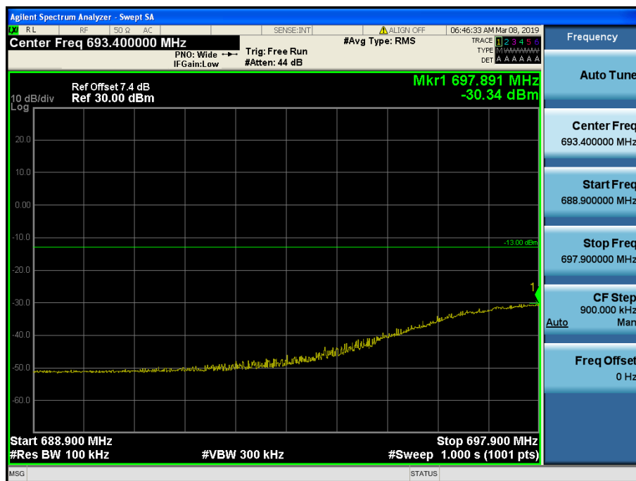
LTE Band 12, 17 / 10MHz / 16QAM - RB Size/Offset (25/0)
