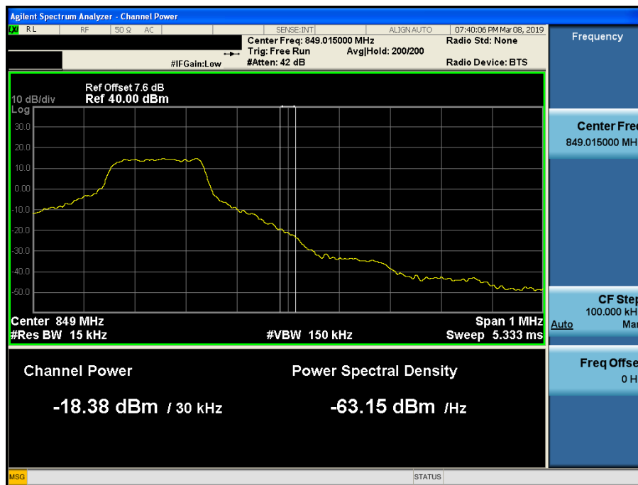
LTE Band 5 / 3MHz / QPSK - RB Size/Offset (1/14)
