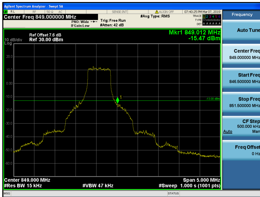
LTE Band 5 / 1.4MHz / QPSK - RB Size/Offset (3/3)
