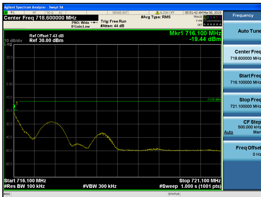
LTE Band 12 / 3MHz / 16QAM - RB Size/Offset (1/14)
