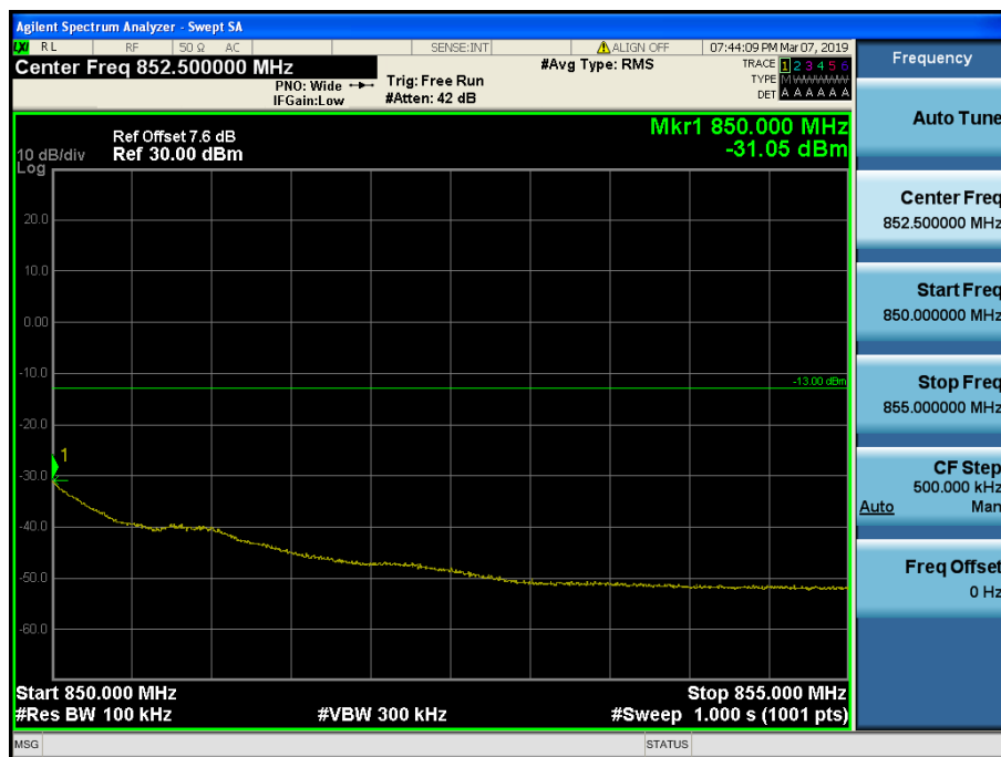
LTE Band 5 / 1.4MHz / QPSK - RB Size/Offset (6/0)
