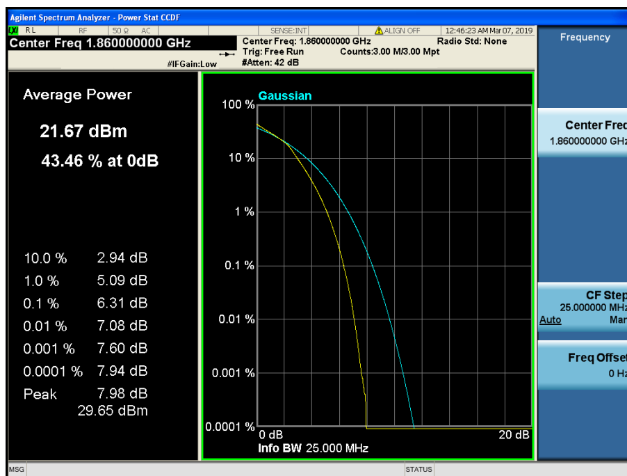
LTE Band 2 / 20 MHz / 16QAM - RB Size 100
