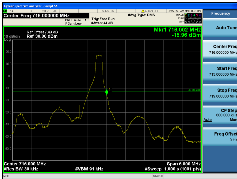
LTE Band 12 / 3MHz / 16QAM - RB Size/Offset (1/14)
