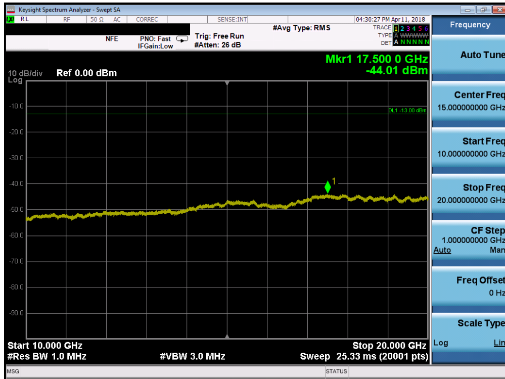
Plot 7-91. Conducted Spurious Plot (Band 2 - 10.0MHz QPSK - RB Size 1, RB Offset 0 - Low Channel)
