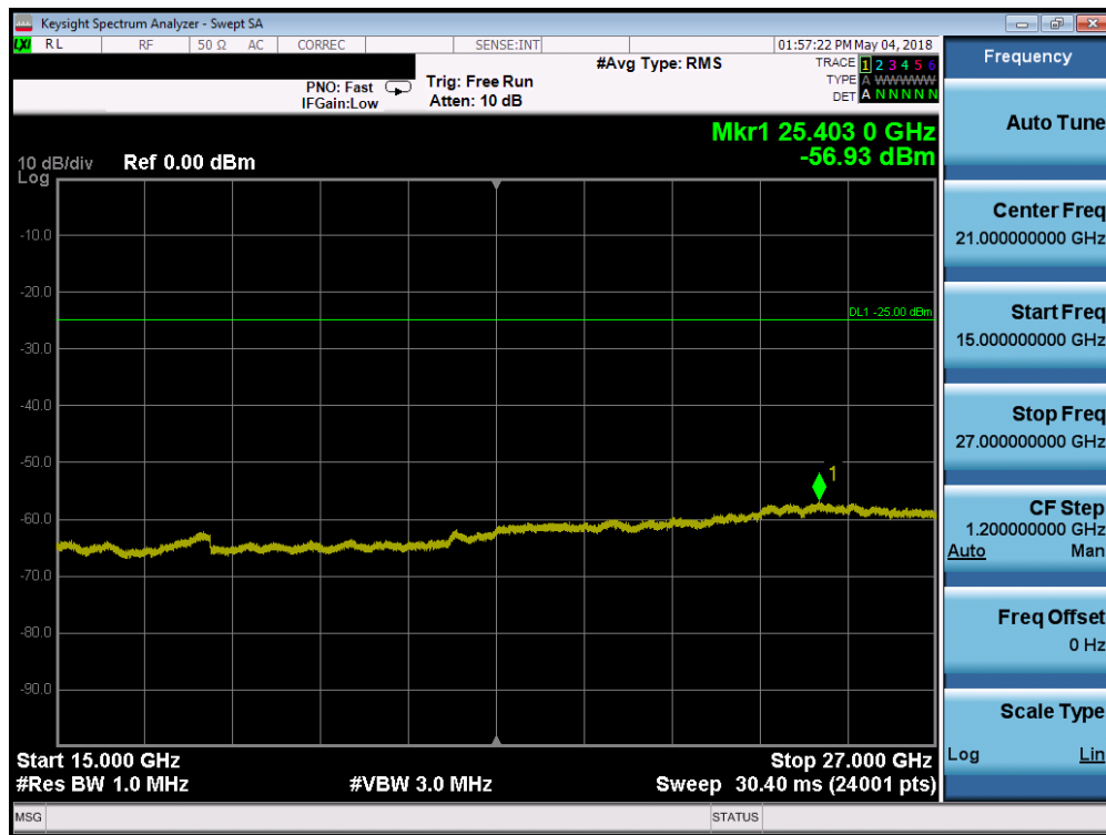
Plot 7-106. Conducted Spurious Plot (Band 7 - 10.0MHz QPSK - RB Size 1, RB Offset 0 - High Channel)
