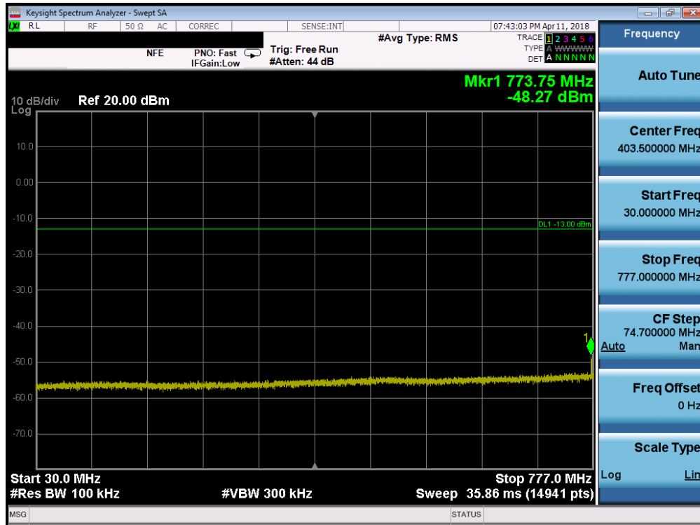
Plot 7-68. Conducted Spurious Plot (Band 13 - 5.0MHz QPSK - RB Size 1, RB Offset 0 - High Channel)
