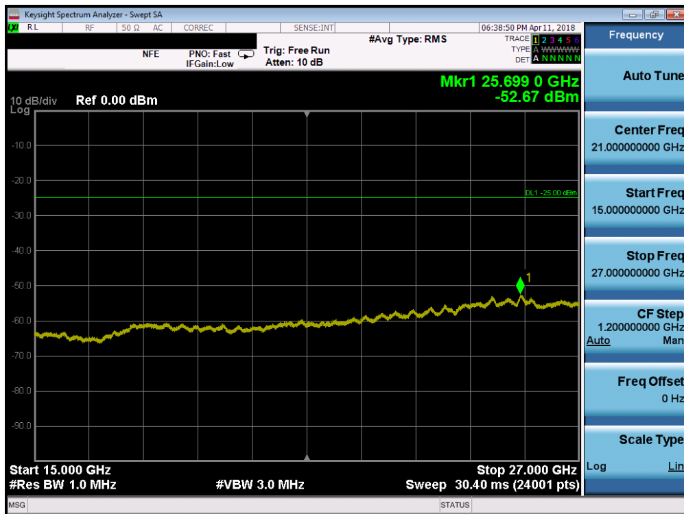
Plot 7-103. Conducted Spurious Plot (Band 7 - 10.0MHz QPSK - RB Size 1, RB Offset 0 - Mid Channel)
