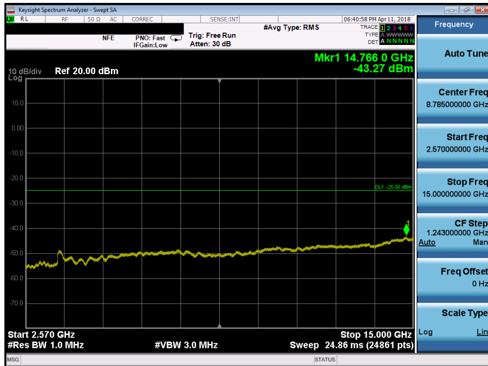
Plot 7-98. Conducted Spurious Plot (Band 7 - 10.0MHz QPSK - RB Size 1, RB Offset 0 - Low Channel)
