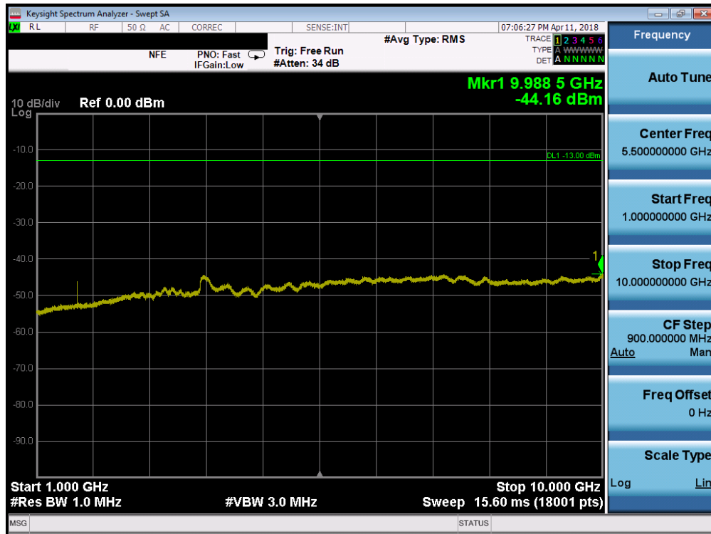
Plot 7-73. Conducted Spurious Plot (Band 5 - 10.0MHz QPSK - RB Size 1, RB Offset 0 - Low Channel)
