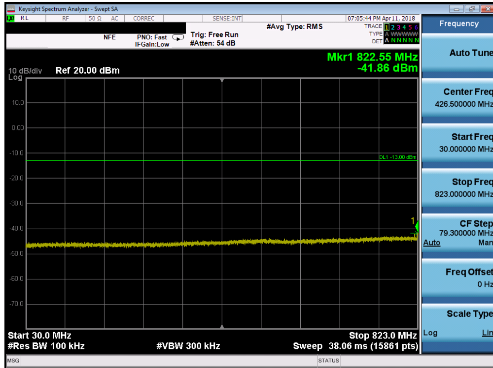
Plot 7-71. Conducted Spurious Plot (Band 5 - 10.0MHz QPSK - RB Size 1, RB Offset 0 - Low Channel)
