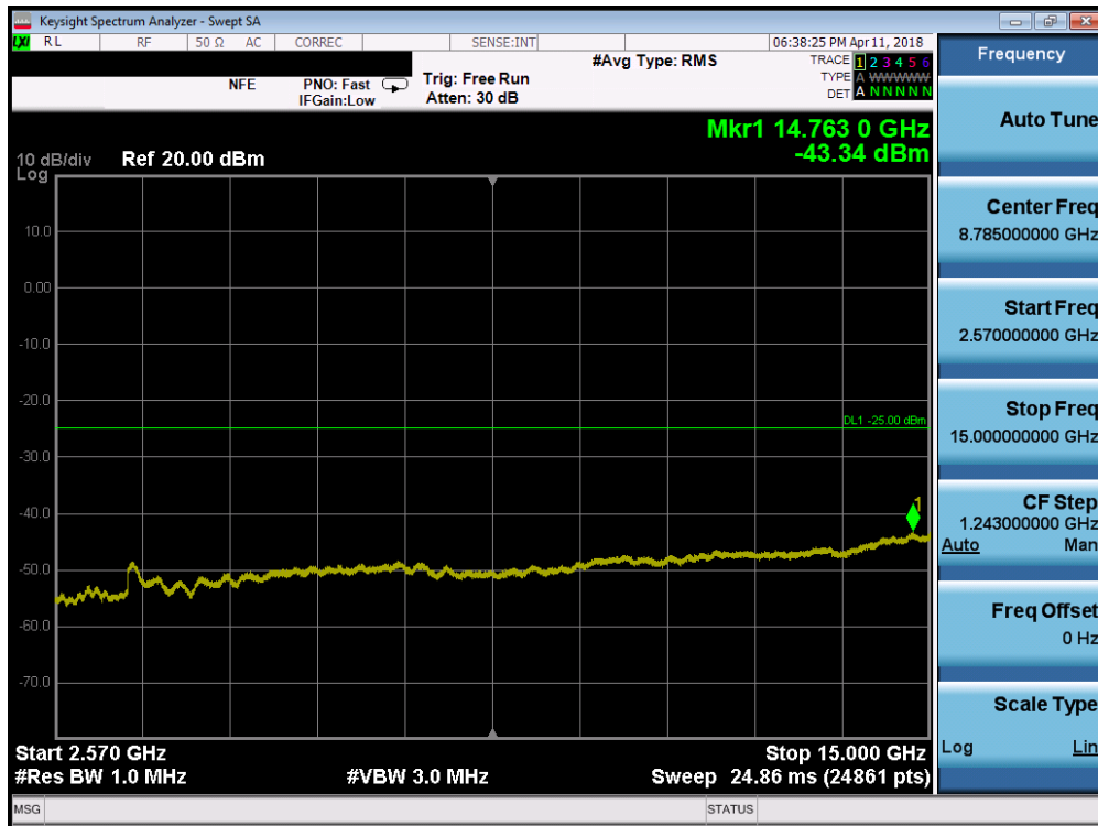
Plot 7-102. Conducted Spurious Plot (Band 7 - 10.0MHz QPSK - RB Size 1, RB Offset 0 - Mid Channel)
