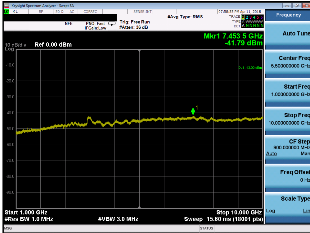
Plot 7-61. Conducted Spurious Plot (Band 12/17 - 10.0MHz QPSK - RB Size 1, RB Offset 0 - High Channel)
