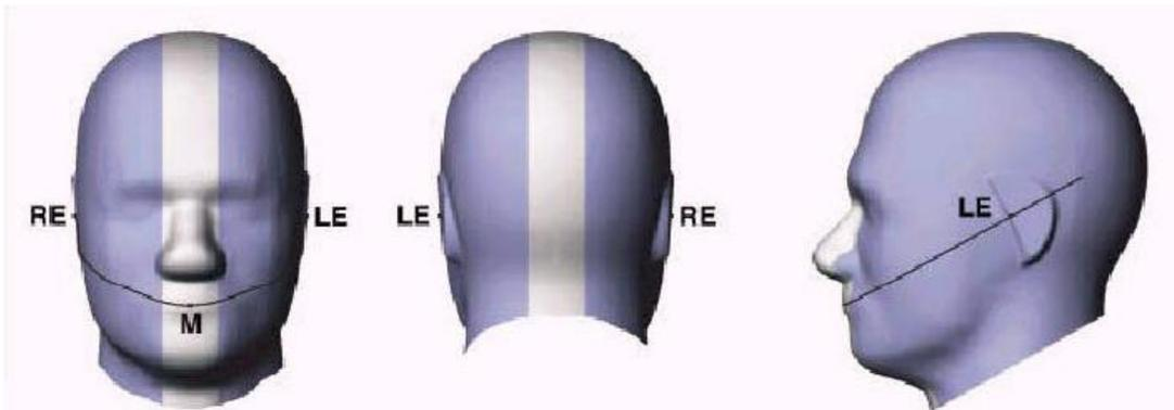
Fig.8.1 Illustration for Front, Back and Side of SAM Phantom
