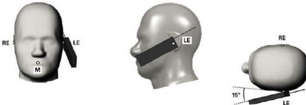
Fig.8.4 Illustration for Tilted Position
