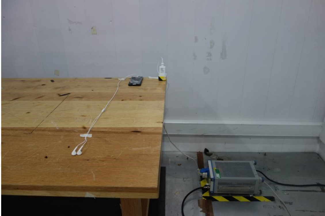
Power Line Conducted Emissions
