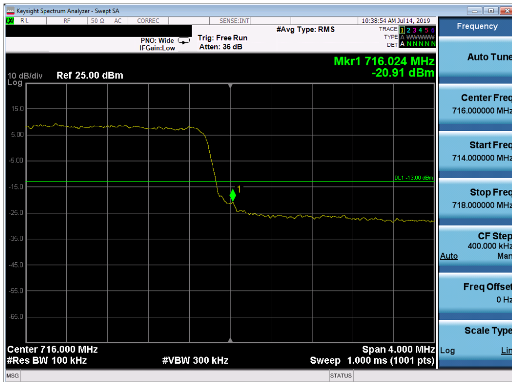
Plot 7-178. Upper Band Edge Plot (Band 12/17 - 5.0MHz QPSK - Full RB Configuration)
