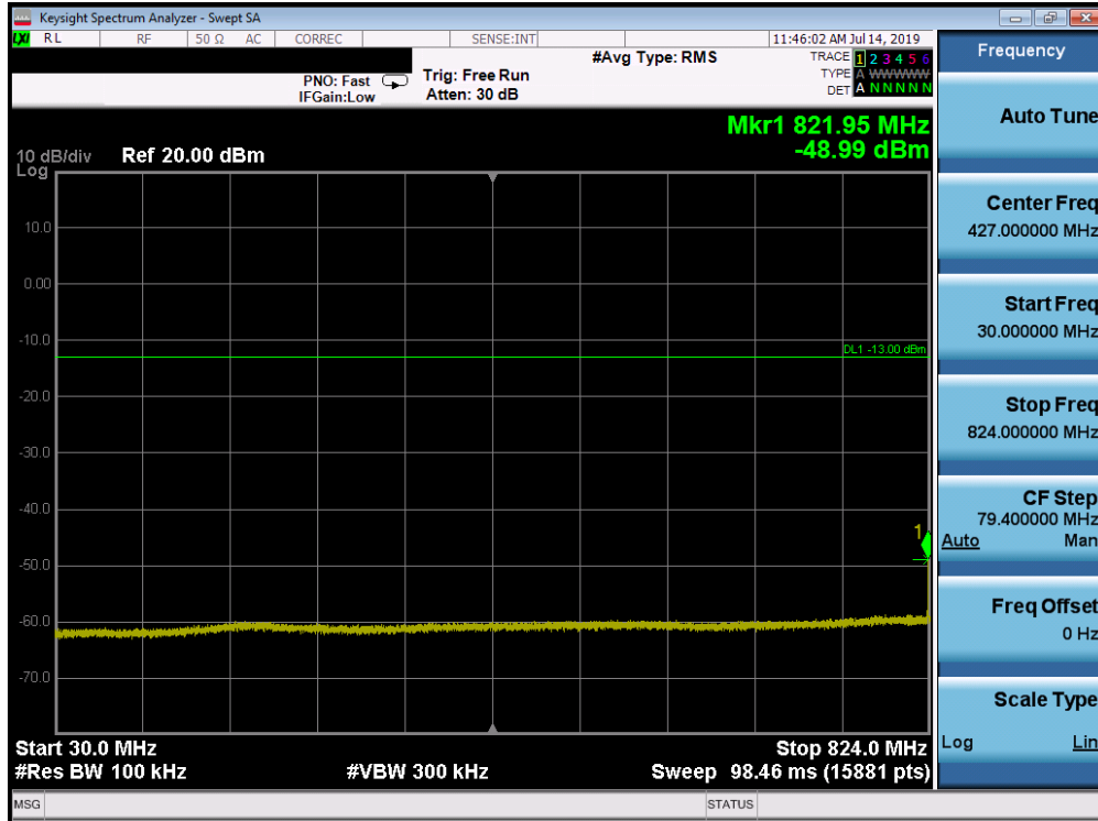
Plot 7-133. Conducted Spurious Plot (Band 26/5 - 10.0MHz QPSK - RB Size 1, RB Offset 0 - High Channel)
