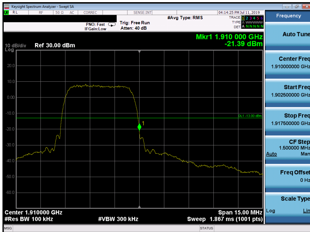
Plot 7-93. Band Edge Plot (PCS WCDMA Mode - High Channel)
