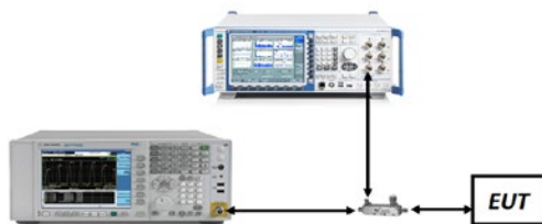
Figure 7-4. Test Instrument & Measurement Setup
